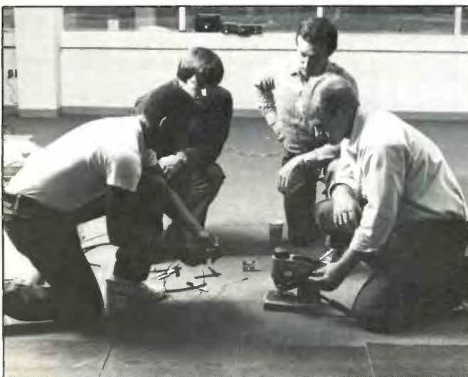
Special tools help simplify installation of fiber-optic cable. When small slitting block is pulled lengthwise over cable, strength members and ramp material are precisely separated from the jacketed optical fibers. A blanking tool is then used to square off the end of the optical fiber.
