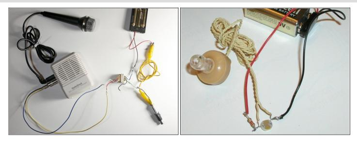
• To send secret voice communications, move the amp from the receiver to the transmitter and plug in a mic. You're ready for the field; just be careful with the volume, to protect the laser.
