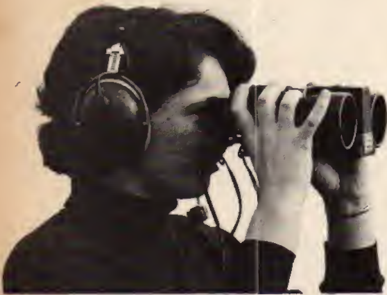
A modified pair of binoculars used as an optical transceiver. The range is about half a mile, but the required power is minimal in comparison to conventional systems
