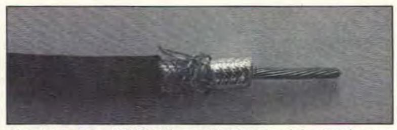
Photo B. A piece of 9096 with an end stripped and the tinned copper braid pulled back to reveal the aluminum-mylar film shield. You would not normally do this to install connectors. That #9 stranded center conductor is a healthy bunch of copper.
