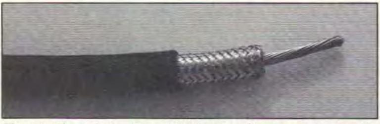
Photo A. The end of a piece of 9096 stripped and ready for installation of a "UHF" PL-259 connector. It strips easily and is a pleasure to work with: One razor blade and five seconds is all it takes to do this.
