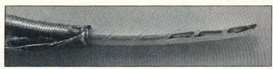
Photo C. A piece of 9096 cut away (sectioned) to reveal its internal construction. If you look closely you can see the spiral turns of polyethylene dielectric, with 1/2" air spaces between them.
