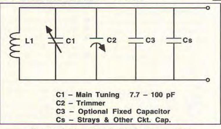
Figure 3. L-C resonant tank circuit for example calculations.
