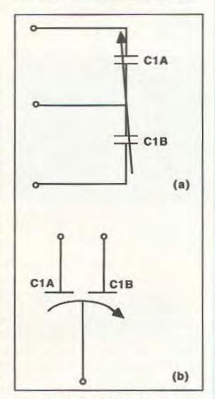
Figure 1. A) Split-stator capacitor symbol; B) Differential capacitor symbol.
