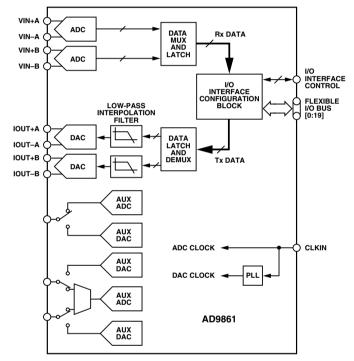
Figure 2. Block diagram of a representative MxFE IC, the AD9861.
