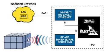
Figure 4. Example of a PoE-based RFID asset-tracking system.
