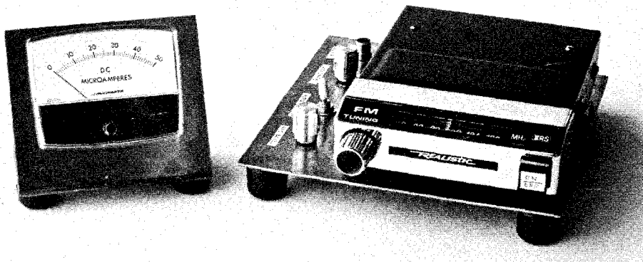
Figure 9-6. Radio Shack FM Converter with AFC & Audio Amps The shielded Level-I communications system Mark II. The Radio Shack 12-1348 FM car converter has built-in AFC; the converter is mounted on two 3 by 6 (77 by 153 mm) G10 double-sided PC boards soldered together to form a baseplate. Microammeter at left is used as an optional S meter.
