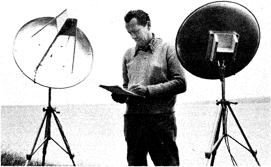
Figure 11-6. Tripod/Mast Mount & 25''D. Parabolic Reflectors
