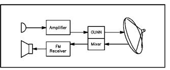
Figure 2—A Gunnplexer station setup. An FM receiver tuned to 30 MHz acts as the receiver.
