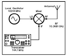
Figure 1—A simplified drawing of a transverter.
