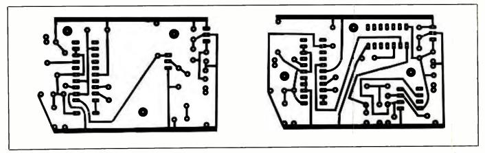
Fig. 5. Actual-size etching-and-drilling guides for the transmitter's (A) and receiver's (B) printed-circuit boards.
