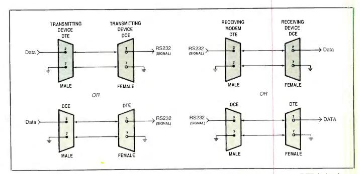
Fig. 9. The RS232 connectors must be wired to be compatible with the equipment they connect to. DTE devices have male connectors and transmit on pin 2. DCE devices have female connectors and transmit on pin 3. Pin 7 is signal ground.
