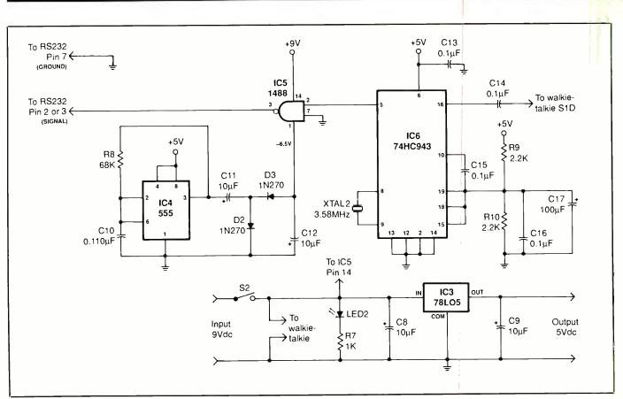
Fig. 4. Schematic diagram of the receiver unit from the output of the walkie-talkie to the RS232 interface.
