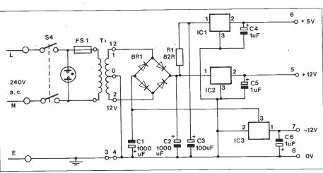
Figure 4. PSU circuit diagram
