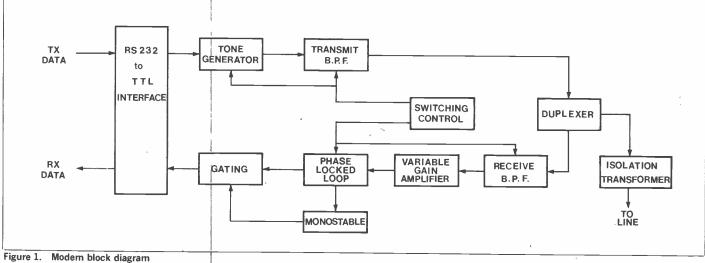
Figure 1. Modern block diagram
