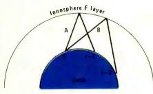
*Figure 1* Showing that high angle signal at A will travel less the distance than the low angle signal at B.
