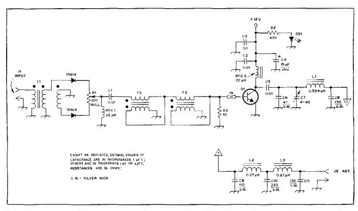
Fig. 1 - Schematic diagram of the transmitting converter. R1 is used to null the 14-MHz signal feedthrough. The low-pass tilter consisting of C9, C10, C11, L2 and L3 is required to reduce the harmonic content in the output signal.
