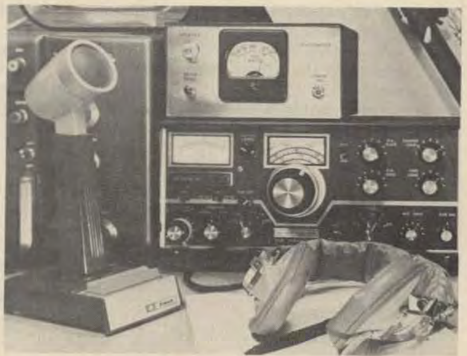
Photo D. Although it fits nicely on top of the transceiver, the Splatmeter can be placed anywhere within the operator's field of view. It doesn't need constant attention; when you splatter, it lets you know with a bright flash.
