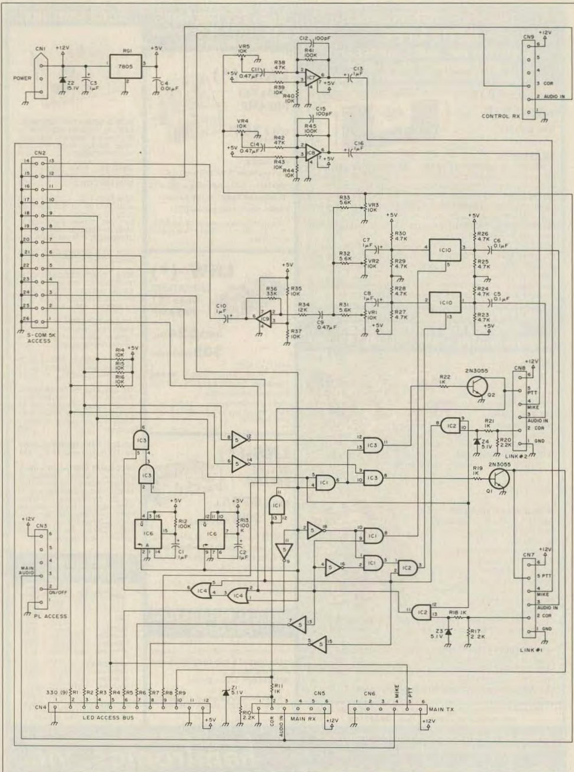
Figure 3. Schematic for the complete board of the 5K link controller.
