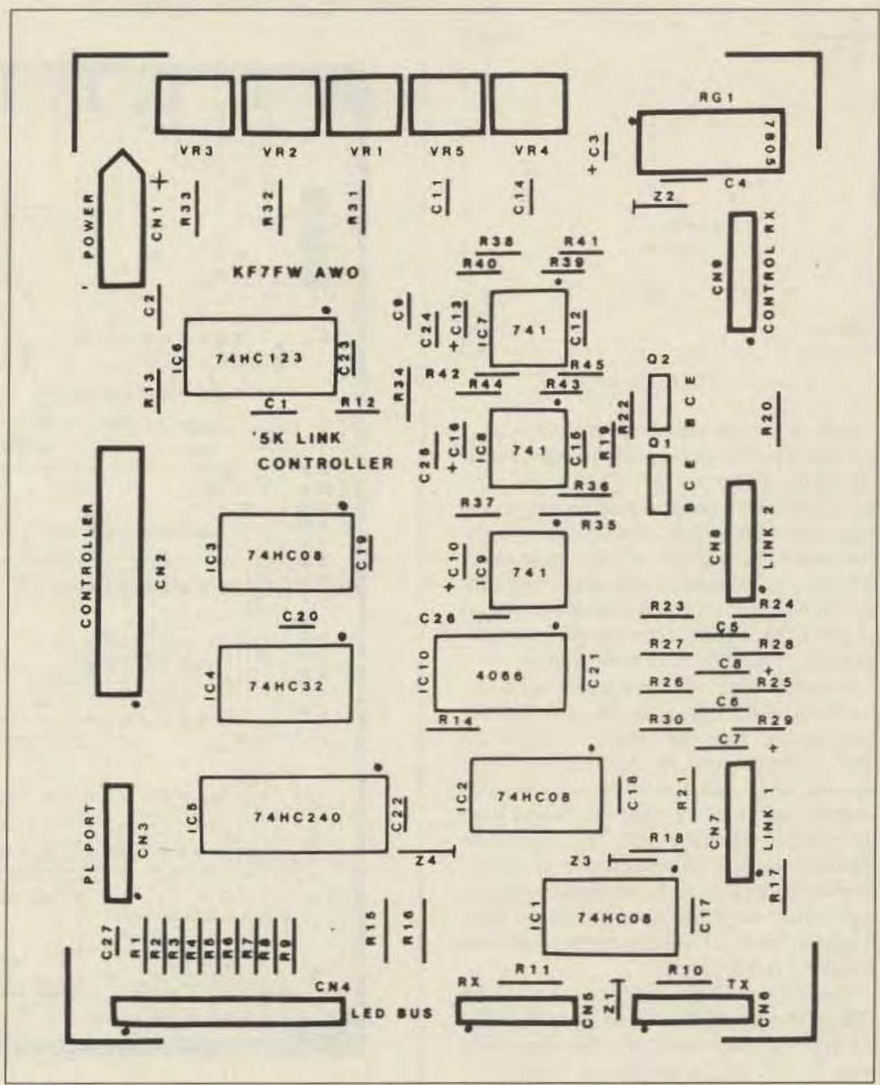
Figure 4. Main board parts layout.
