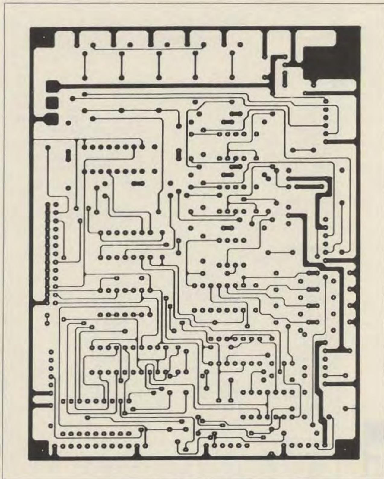
Figure 6b. Bottom foil layout for the main board.
