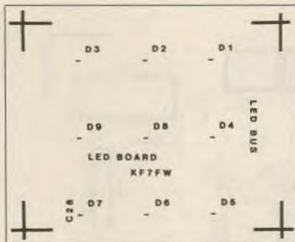
Figure 5. LED board parts layout.
