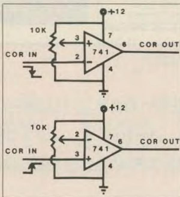
Figure 2. Receiver COR circuit.
