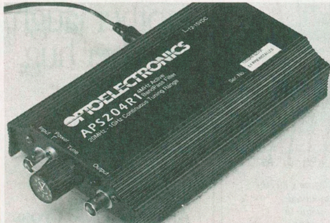
The Optoelectronics APS-204 six-octave, tunable, bandpass filter maintains a constant 4-MHz bandwidth over a range of 20 to 1000 MHz.
