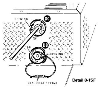
Position pulleys DC and DB with their openings as shown in Detail 8-15F.
