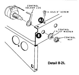
control nut. Form the control solder lug against terminal 1 of the control. Before soldering, check to see that the formed lugs will fit under the chassis lip at R. Solder lug 1 (S-1), and then remove the control flat washer and control nut.
