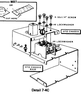
Refer to Detail 7-4C and mount the variable capacitor at FB on the VFO chassis as directed in the following steps.
