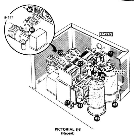
( ) Refer to Detail 8-8B and cut 5/8" from the long end and 1/4" from the short end of the 10 meter final tank coil (#40-549).
