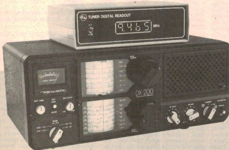
The Tuner Digital Readout can be used with broadcast-band AM tuners and communications receivers.
