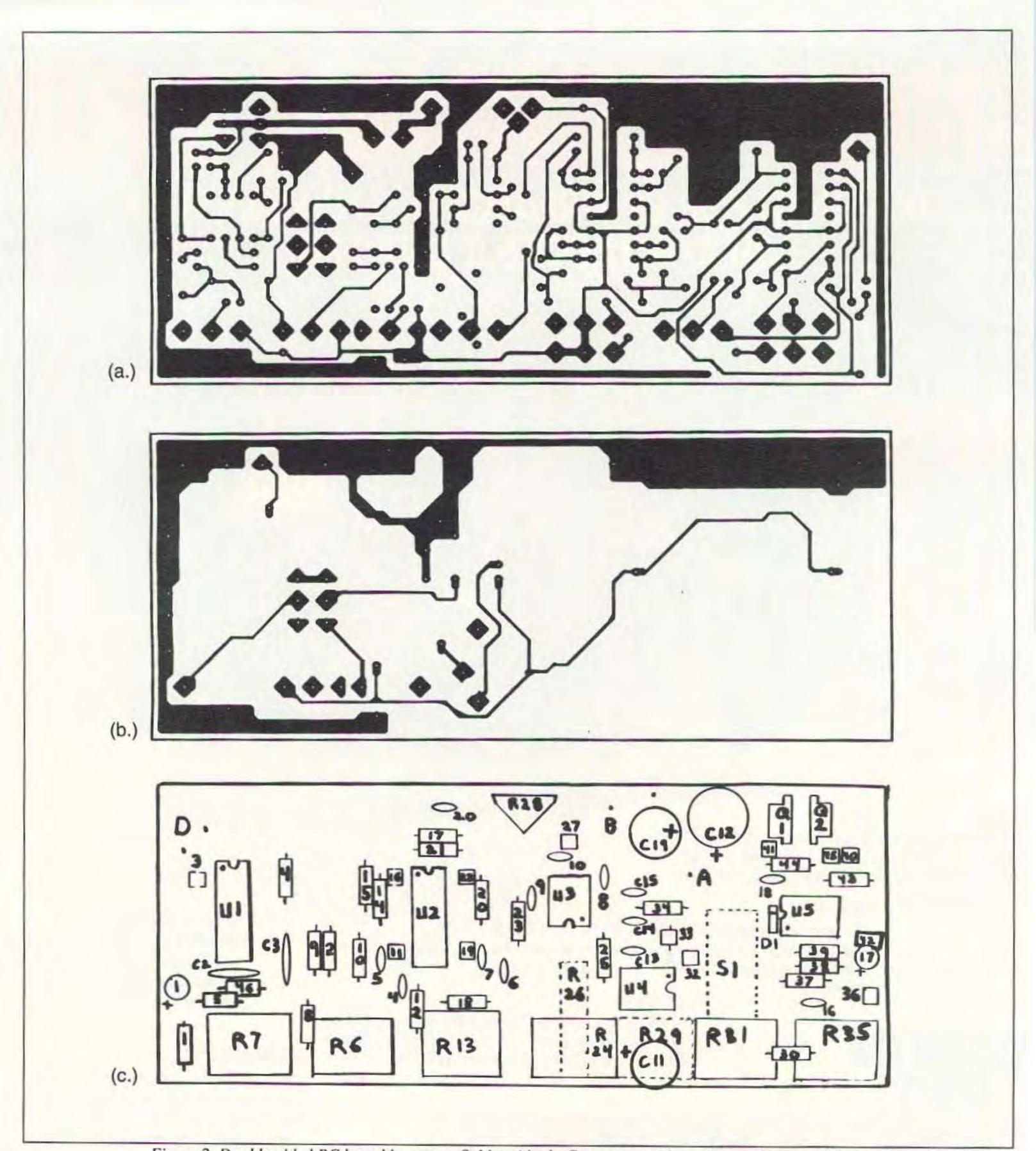
Figure 2. Double-sided PC board layout: a. Solder side; b. Component side; c. Parts placement diagram.
