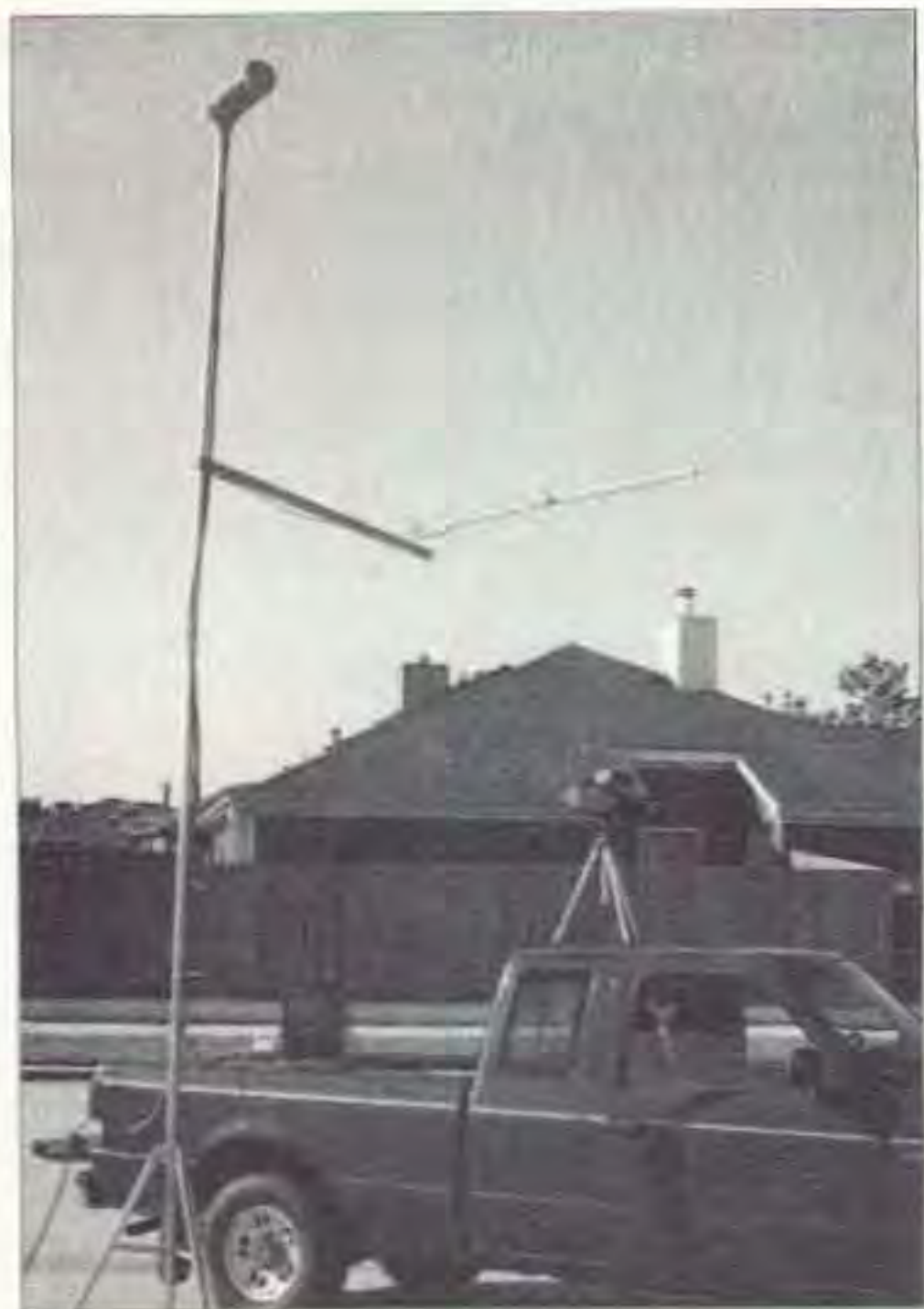
Photo D. Portable system configuration used during this year's March of Dimes Walkathon. Note Delta board to left of TV, above rear wheel.
