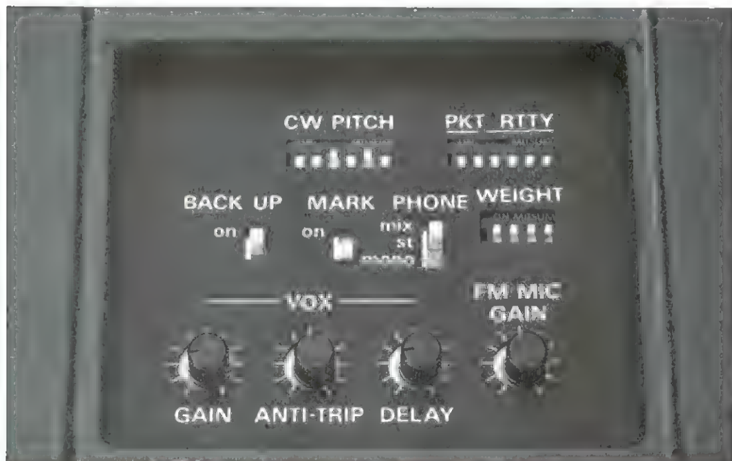
Figure 2.5 — VOX controls — Gain, Anti-VOX (called Anti-Trip on this transceiver) and Delay. Because they aren't often adjusted, many rigs place manual Gain and Anti-VOX controls out of the way. They are menu items if controlled by software. Delay is adjusted most often and is usually made the easiest to access by a front-panel control. Some radios even have separate Delay controls for CW and phone.
