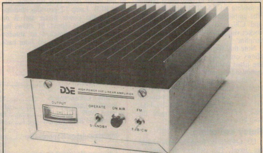
View of the completed prototype. The large finned heatsink allows the amplifier to be operated continuously at full output.
