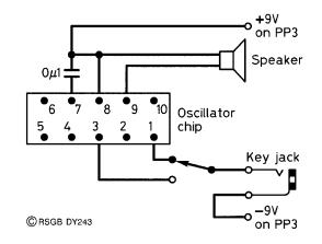
Figure 1 Morse oscillator, circuit diagram
