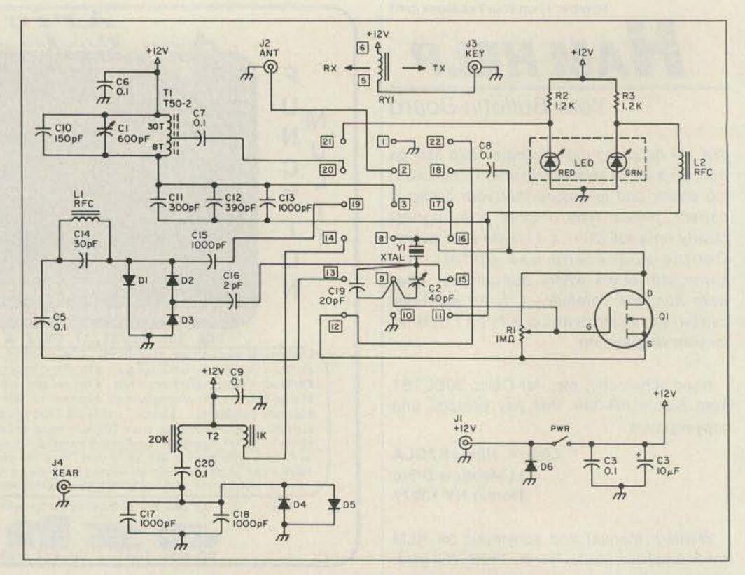
Figure 1. Schematic of the WB3ELL DMOS 80 meter CW transceiver.
