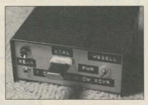
Photo A. The completed DMOS 80 meter CW transceiver.
