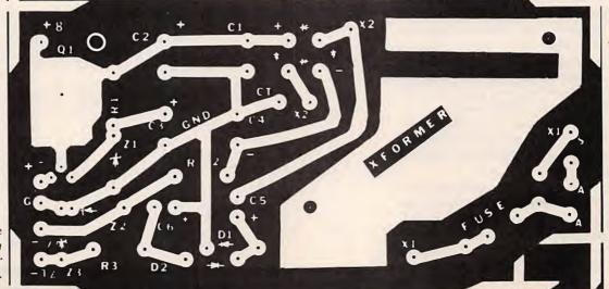
Fig. 9. Actual-size etching and drilling guide for the power supply board.
