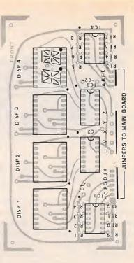
Fig. 8. Parts placement guide for front side of display board is above.
