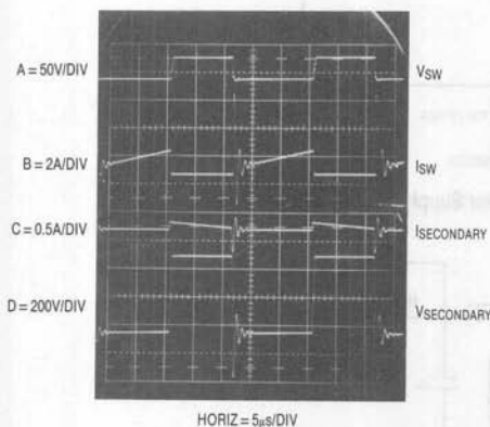
Figure 3. Operating Waveforms for High Voltage Converter
