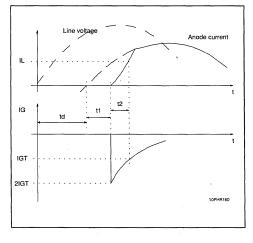
If the phase lag is not constant a gate pulse train can be used, the calculation parameters are the same, except for R2 : the capacitor C has to be charged between 2 pulses so the equation is :
