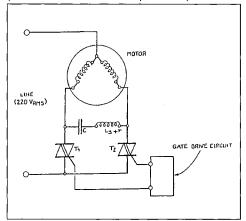
2. Motor drive circuits. Figure 11 shows an inversion circuit of an asynchronous motor where spurious firing of the triac, normally assumed to be in off- state, must be absolutely be avoided.
