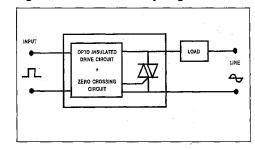
Figure 11: Motor control circuit using SNUBBERLESS triacs
