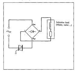
Circuits which generate wave forms with a very high (di/dt)c, such as inductive load supplied by a diode bridge (fig. 13). It is only limited by the parasitic inductance of the AC circuit.
