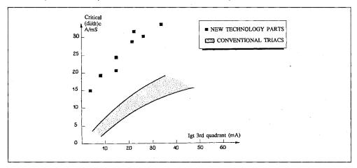
The new technology has been put into place with the manufacturing of the two new series, Logic Level and SNUBBERLESS Triacs. In the data sheets of these new triacs a critical (di/dt)c limit is specified at the maximum junction temperature (Tj max).
