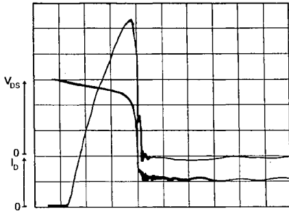
Figure 12 : Turn-on Illustrations of the MOSFET Drain to Source Voltage ( V_{DS} ) and Current ( I_D ) at Turn-on of the Transistor Limited to 100A/ \mu s.
