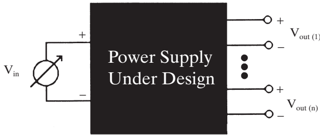
Figure 3–17 The SMPS treated like a black box.
