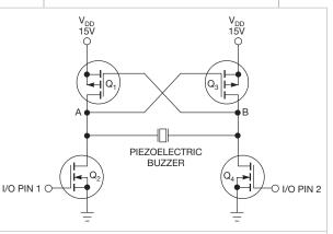
Figure 1 This cross-coupled configuration enables you to drive a piezoelectric buzzer from a microcontroller's I/O pins.
