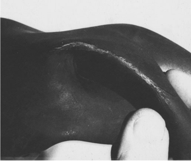
FIGURE 2.28 Age cracks. (Courtesy ASTM.)
