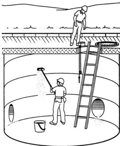
FIGURE 7.9 Vault atmosphere monitoring.
