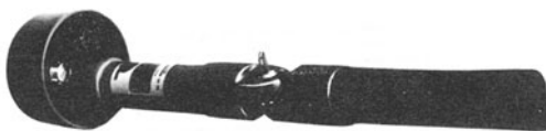
FIGURE 2.46 Voltage tools attached to a hot stick. (Courtesy W.H. Salisbury and Co.)
