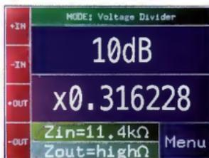
Fig.9: in divider mode, the division ratio can be entered in multiple ways; in this case, in decibels (dB). The attenuation factor is shown below.
