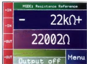
Fig.10: the resistance reference mode is somewhat limited; the selected resistance is shown at the top while the actual resistance is shown below.
