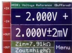
Fig.7: the unit has now been set as a 2V voltage reference with buffered output but the output has not been switched on yet, as shown at bottom.
