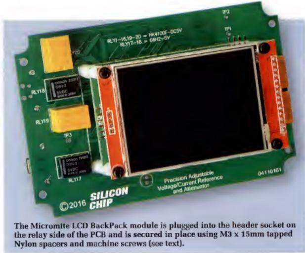
The Micromite LCD Backpack module is plugged into the header socket on the relay side of the PCB and is secured in place using M3 x 15mm tapped Nylon spacers and machine screws (see text).
