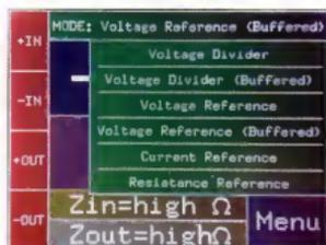
Fig.5: after touching the bar at the very top of the screen, you can select from the six different modes shown here.
