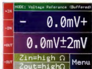
Fig.4: assuming everything is working properly, this is what should appear on the LCD when the unit is first powered up.
