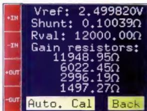
Fig.12: the calibration screen after pressing the Automatic calibration button. Note that the PGA resistors are now shown with the measured values.
