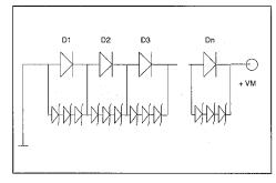
TRANSIL operates as a voltage limiter at steady state, during the switching phase, and also in case of external voltage transients.
