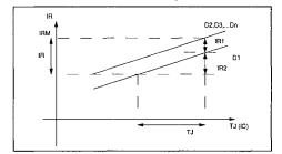
The junction temperature is given by the thermal resistance junction to ambient Rth (j-a) and the power dissipation due to the conduction losses (PC) and the switching losses (PS).
