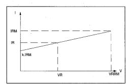
So the leakage current  $I_{\hbox{\scriptsize PM}}$  of diodes D2 ... Dn under the blocking voltage V2 ... Vn is :
