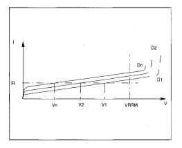
In order to equlize the voltage, a resistor is connected across each diode (Fig.2).
