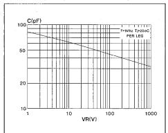
When D1 has evacuated all its stored charge it is equivalent to a capacitor CJ1 and the other diodes D2, D3 ... Dn are equivalent to a capacitor which is the sum of the junction capacitance CJ2, CJ3 ... CJn and the capacitance
