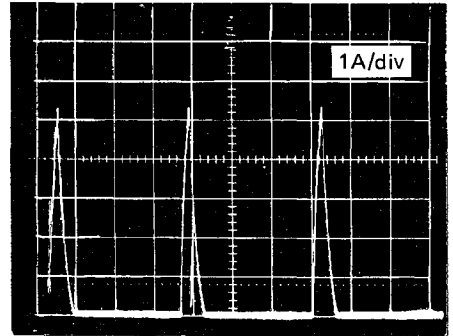
Figure 10 : Load Current in Short Circuit Conditions ( V_i = 40V , L = 300\mu H , f = 100KHz ).
