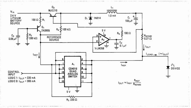
**Injecting current.** Switching source delivers constant current to members of low-power I<sup>2</sup>L logic family without wasting much power. Small reference current, C-MOS switches, and low-power oscillator contribute to circuit efficiency. Two-level current source, which generates up to 300 milliamperes at 2.3 volts, can provide one of five current values if additional programming inputs are introduced at switch A<sub>1</sub>.
