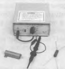
Figure C3. Typical Current Shunts and an "Isolated" Probe
