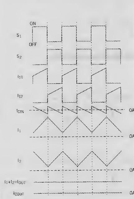
**Figure 3** Interleaving reduces input-capacitor rms current ( $I_{CIN}$ ) and output-capacitor ripple current ( $I_{COUT}$ ).
