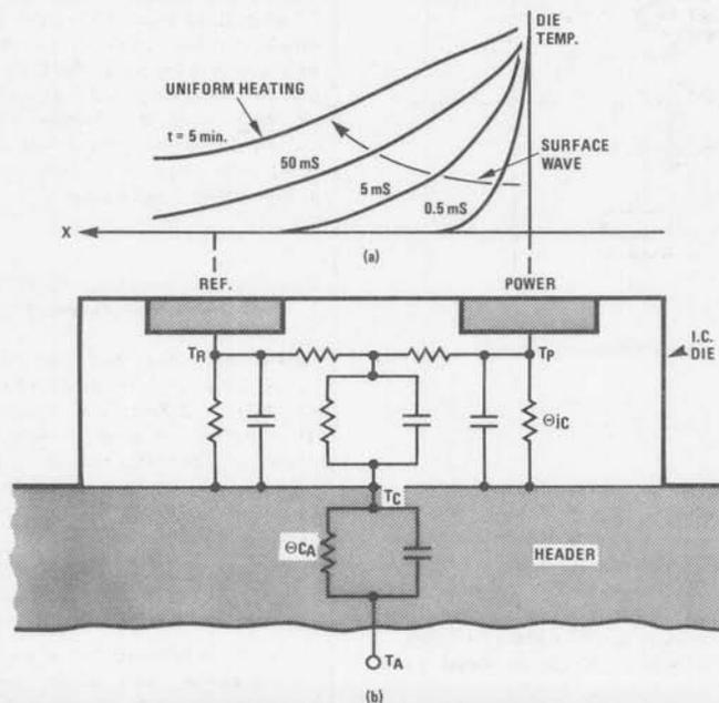
FIGURE A3.7(a). Plot of Die Temperature vs. Distance (x) Along Die After Power Transistor is Turned On.
