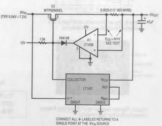
Figure 2. Ultra-Low Dropout Regulator
