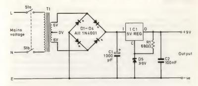
Figure 11.2 Circuit diagram of the adapter
