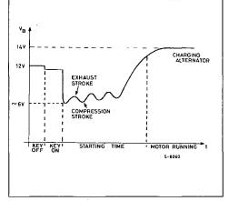
Figure 1 : Cold Starting Supply Voltage Drop.
