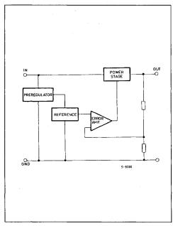
Figure 8 : Block Diagram of L387A and L487 Series Regulators.
