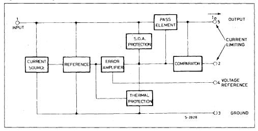
Figure 2 : Schematic Diagram.
