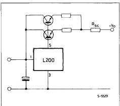
VOLTAGE REGULATOR FROM 0 V TO 16 V - 4.5 A
