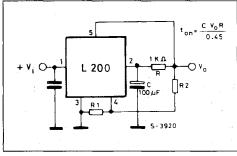
Capacitor C is charged by the constant current ic.
