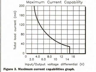
The various performance aspects of the RC4195N regulator IC are detailed in the graph plots, see Figures 1 to 6. The  $\pm$ 15V Regulator Kit is built onto a compact, single-sided board, connections being made via onboard terminal blocks. Provision is made for accurate balancing of the output rails with a negative rail trimmer, and for optional power on indication.
