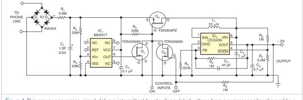
Figure 1 This power-conversion circuit delivers intermittent bursts of regulated voltage from a supercapacitor charged by a trickle of current from a telephone line.
