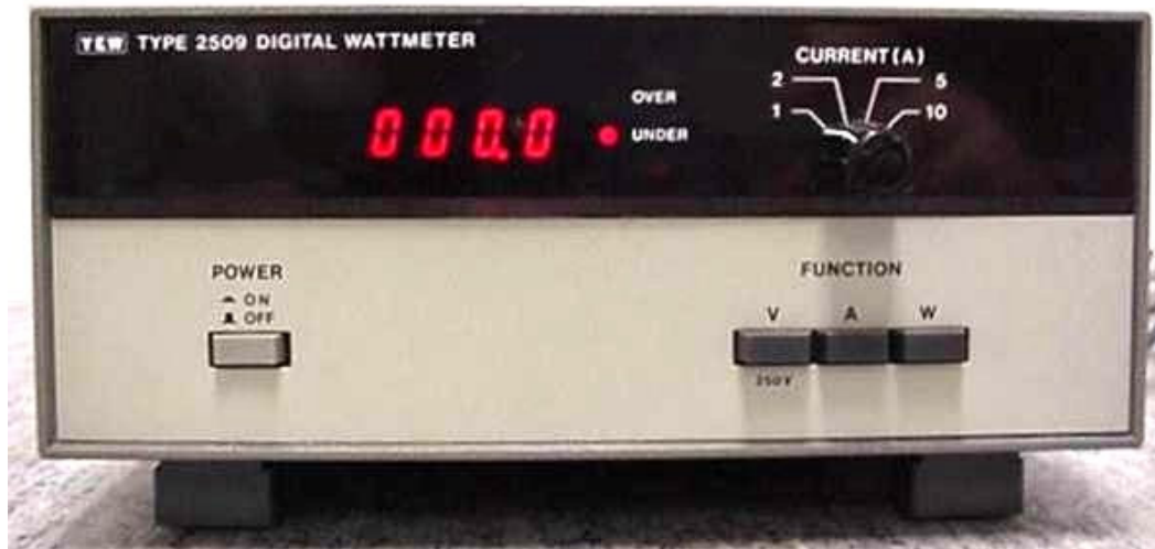
Power Meter Used for Testing
