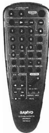
THE OUTPUT OF THIS remote control was "swamped" by an energy-efficient fluorescent tube.
