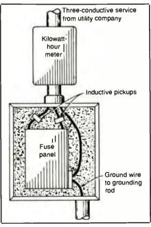
Fig. 4. Pickups must be positioned on insulated wires coming from utility company kilowatt-hour meter, before fuse panel.
