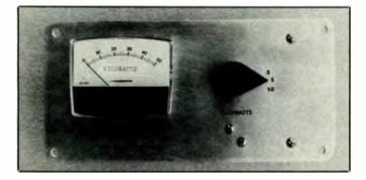
Inductive-pickup meter monitors instant ac power usage so that you can more efficiently manage energy consumption
