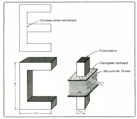
Fig. 2. Inductive pickups are built around laminations salvaged from a small power transformer.
