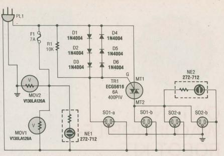
Fig. 3. This circuit for the Socket Sentinel looks odd, but it works very well. The diodes provide the Triac gate with a voltage-limited gate signal.
