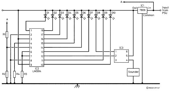
Figure 1 PSU monitor, circuit diagram
